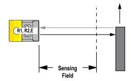
A reflective background object in this position or moving across the sensor face in this axis is ignored.
