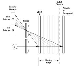
Figure 2. Adjustable field sensing concept
