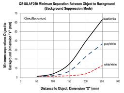
Figure 5. QS18LAF250 minimum separation between object and background
