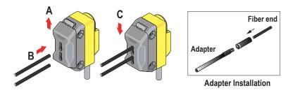
Figure 2. Installing Plastic Fibers
