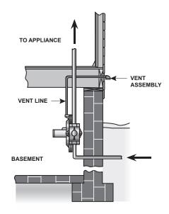
Figure 3. Typical Vent Line Installation
