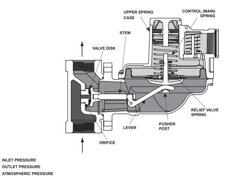
Figure 2. Type HSR Pressure Regulator Operational Schematic
