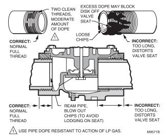
Fig. 4. Preparing the pipes.
