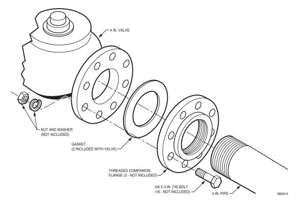
Fig. 6. Installing a 4 in. V5055 Valve.
