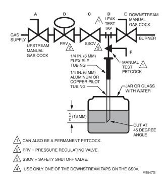
Fig. 7. Valve leak test.
