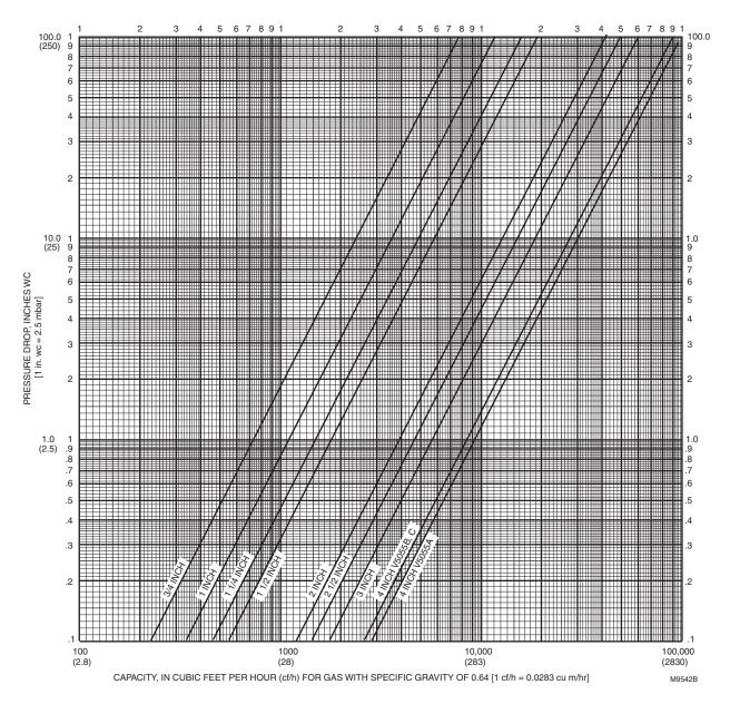
Fig. 1. Flow curves for V5055 Valves.
