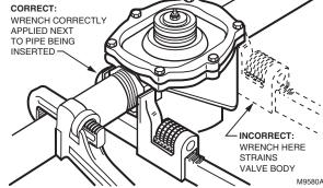
Fig. 5. Installing a 3/4 through 3 in. V5055 Valve.
