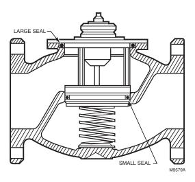
Fig. 9. Proper positions of valve and bonnet seals in 4 in. valves.
