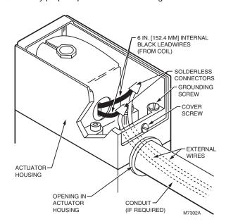
Fig. 12. Wiring connections and actuator housing.
