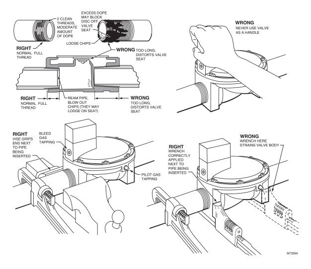
Fig. 3. Preparing piping and installing valve.
