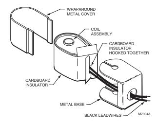
Fig. 15. Coil assembly, insulator, and cover.
