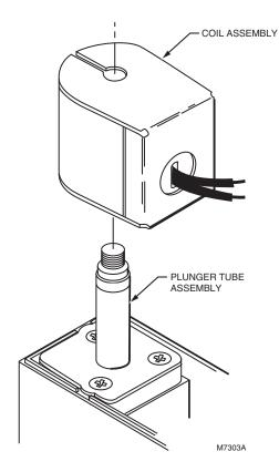
Fig. 14. Coil assembly fits on plunger tube assembly.
