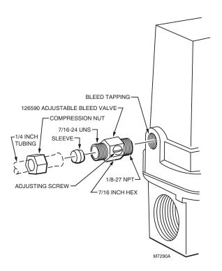
Fig. 8. Installing optional 126590 adjustable bleed valve.
