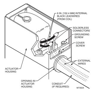
Fig. 7. Making wiring connections.
