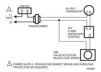
Fig. 6. Typical wiring diagram for V88.
