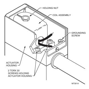
Fig. 13. Internal view of actuator housing.
