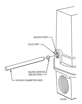
Fig. 9. Installing optional bleed orifice.
