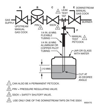
Fig. 16. Valve leak test.
