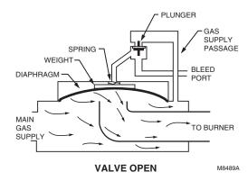
Fig. 10. Operation of V48 and V88 diaphragm gas valves.
