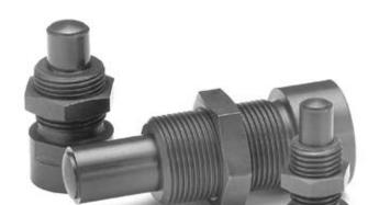
With side load impact angles of more than 3° the operating lifetime of the shock absorber reduces rapidly due to increased wear of the rod bearings. The optional side load adapter provides a long lasting solution.
