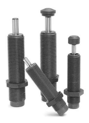
SC² 300 and SC² 650 Heavyweight Series Shock Absorbers deliver up to 950% of the effective weight capacity and 280% of the energy absorption capability of standard models. These durable units are ideal for decelerating heavy weights moving at low velocities. The Heavyweight Series design combines the piston and the inner tube into a single component, the piston tube. It acts as both the pressure creating and pressure controlling device.
